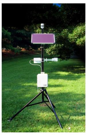
The HazMET100 Portable AWS is an advanced, Portable Automated Weather Station built around the 2100-138 Multi-parameter Meteorological Sensor. The low power requirements of the HazMET100 AWS make it well suited for portable battery and solar powered applications. The system has been designed from the ground up for fast setup anywhere.
